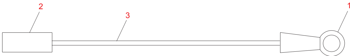
Figure 3-81: Ignitor to Relay Cable Assembly
